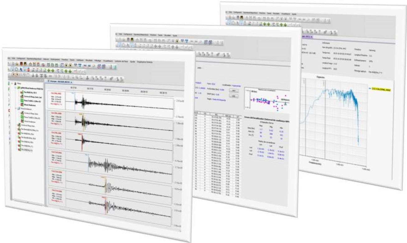
Figure 7.7: Posidó interface for hypocentral location, magnitude calculation and signal processing.
