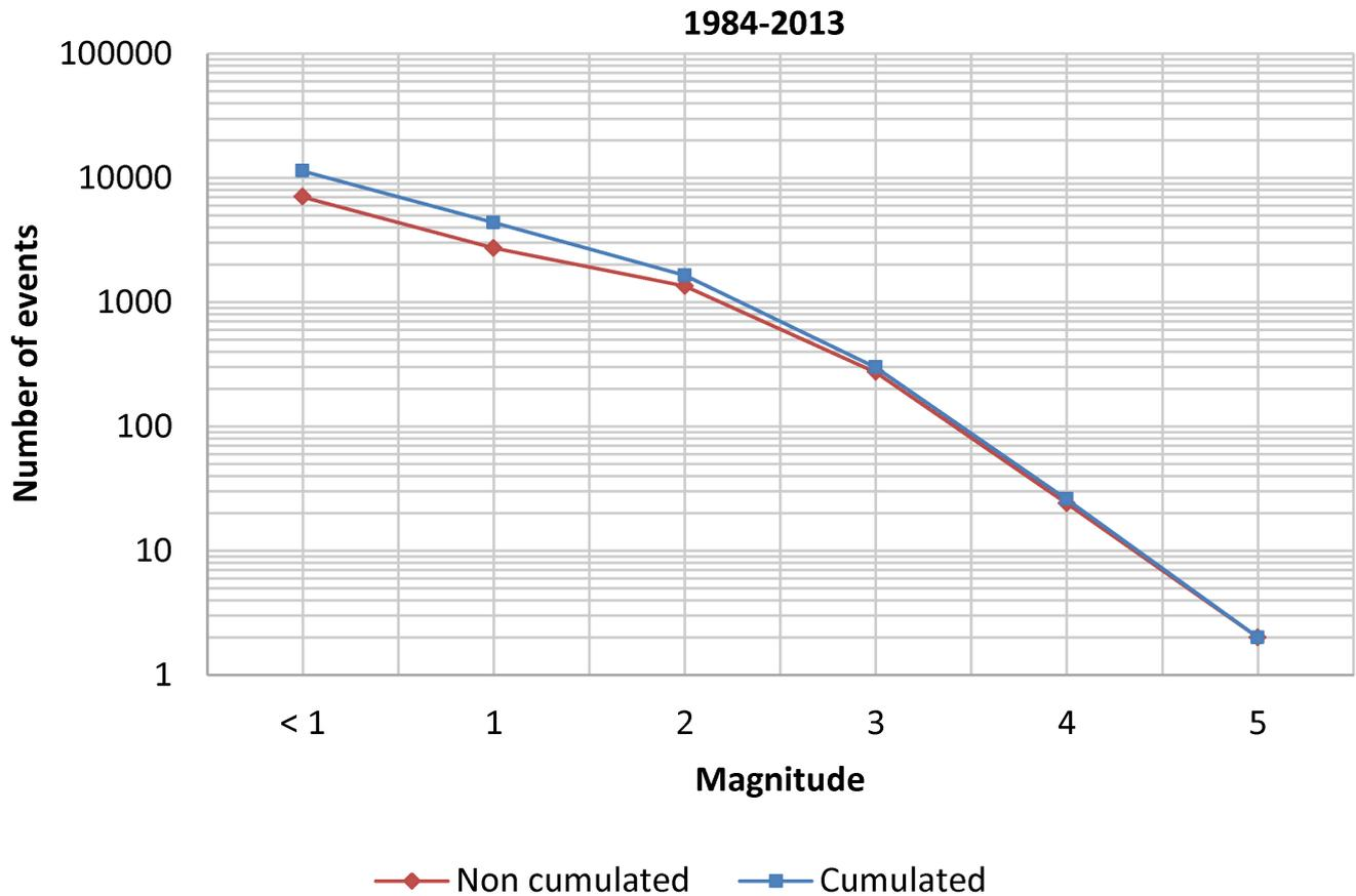
**Figure 7.2:** Gutenberg-Richter relation for the seismic events that occurred in Catalonia for the period 1984-2013.
