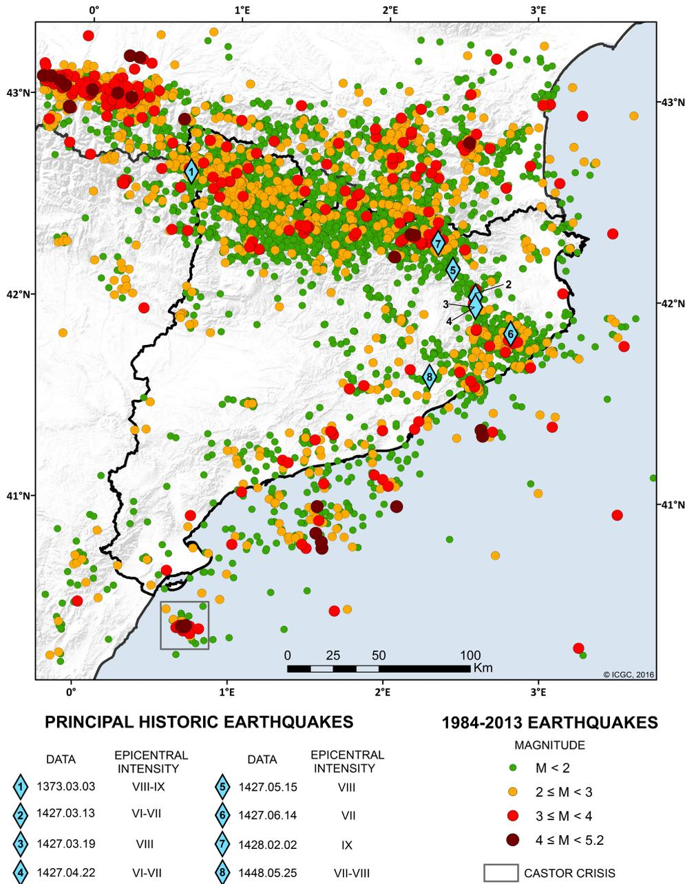
**Figure 7.1:** Instrumentally recorded seismicity for the period 1984-2013 (dots) and the main historical events (diamonds). The small square in the SW part is the place of the CASTOR crisis induced seismicity episode and it accumulates hundreds of events.
