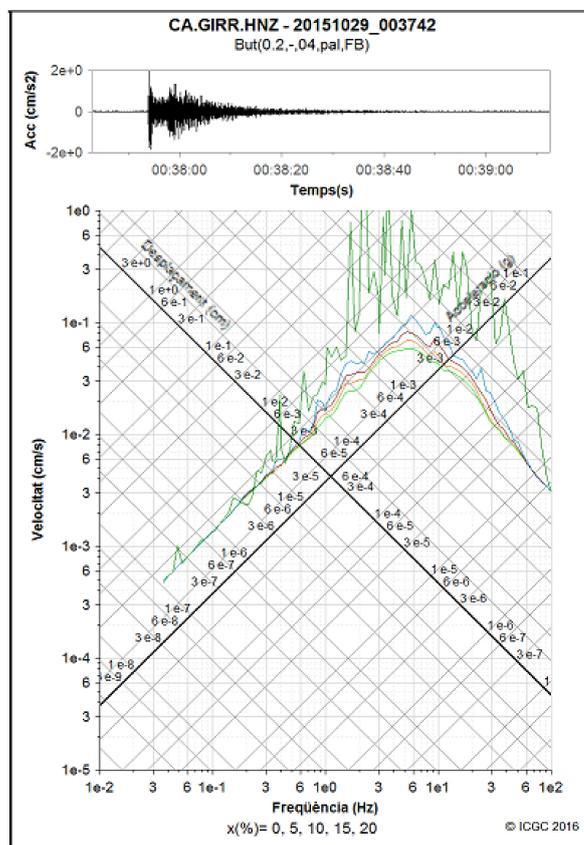
*Figure 7.11: (Left) Table of acceleration records and (right) an example of accelerogram and elastic response spectrum at different damping values.*
