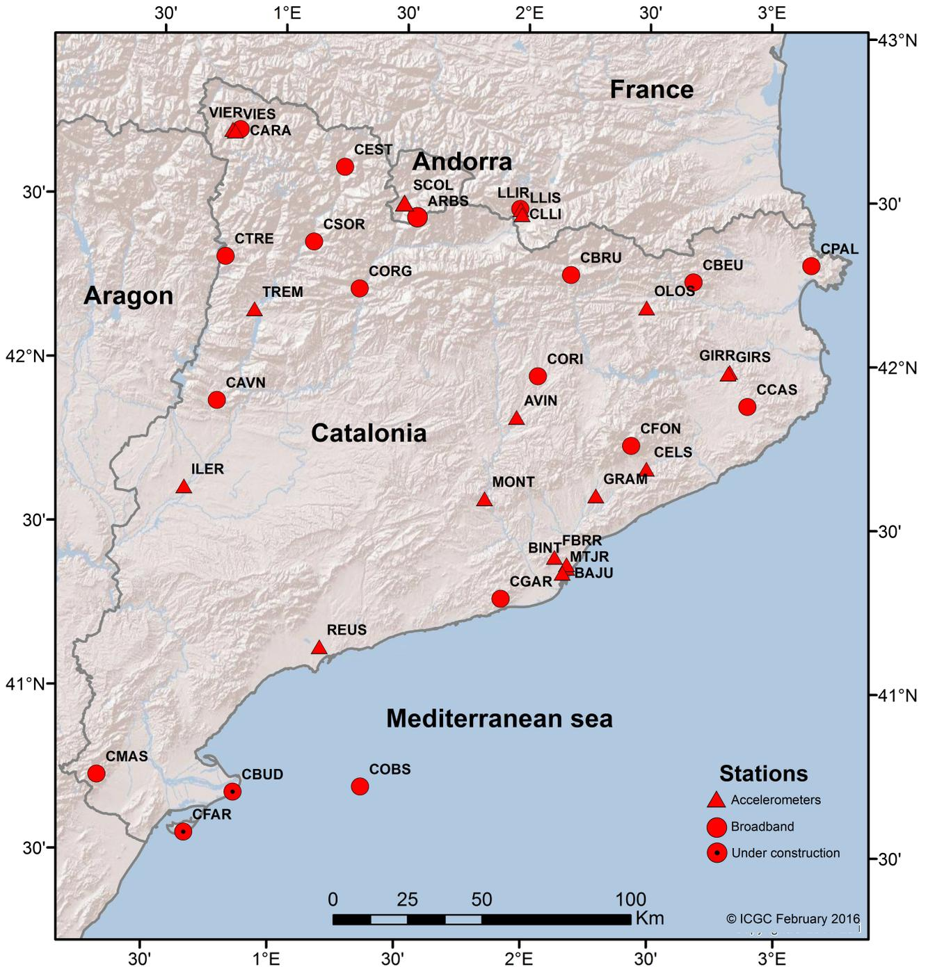
**Figure 7.3:** Distribution of broadband and accelerometric stations operated by ICGC. Stations SCOL and ARBS are jointly operated by ICGC and IEA.
