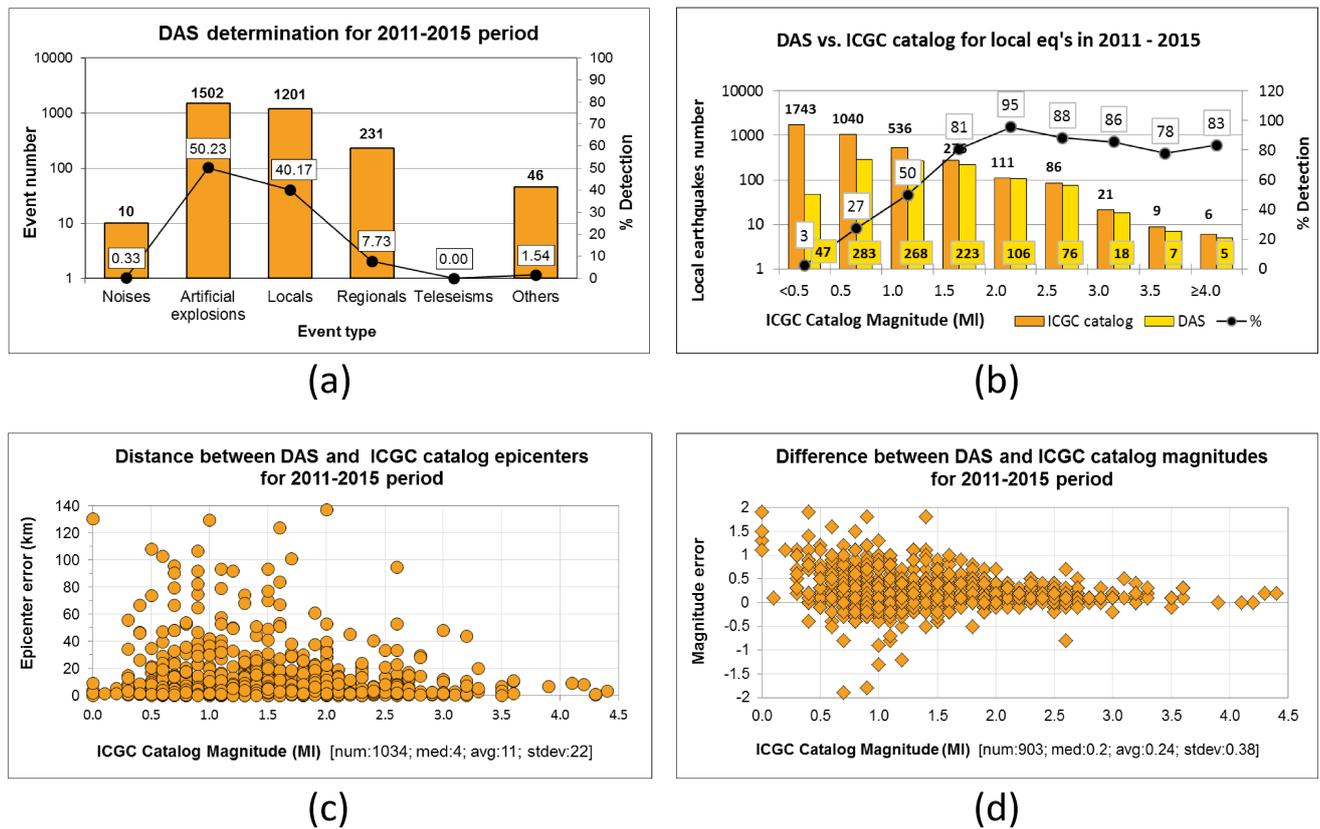
**Figure 7.4:** DAS performance results for 2011 – 2015 period. (a) DAS determination classified by event type. (b) Comparison between local earthquakes detected by DAS and ICGC catalogue. (c) Location error of local earthquakes detected by DAS. (d) Magnitude error of local earthquakes detected by DAS.
