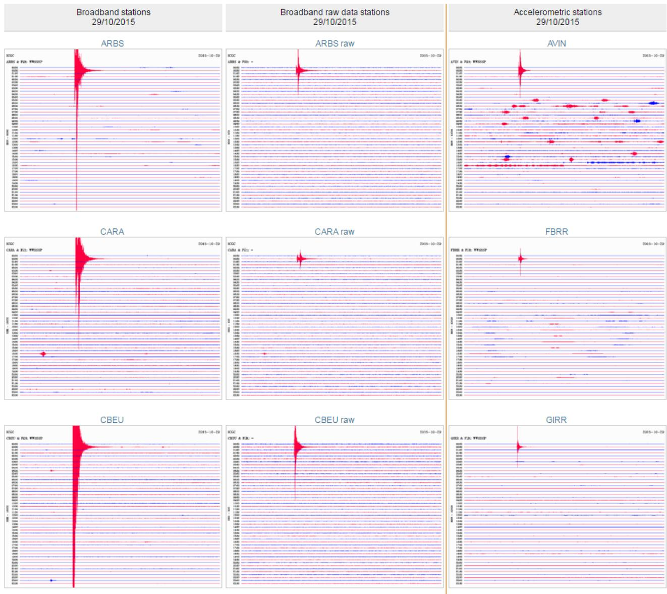
**Figure 7.12:** Example of the seismic live data service for the M4.3 earthquake in the Roses Gulf that occurred on October 29th, 2015. All day long waveforms are shown for 4 broadband stations (ARBS, CARA, CBEU, CFON): filtered (left column) and in raw format (centre column); also 3 accelerometric stations (FBRR, GIRR, GRAM) are shown (right column).
