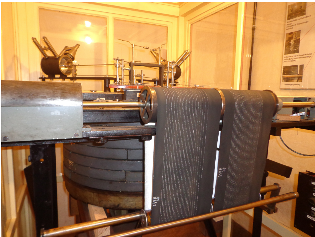
Figure 5.3: Wiechert seismograph still working in seismometer hut (Petra Buchholz, 2017).
