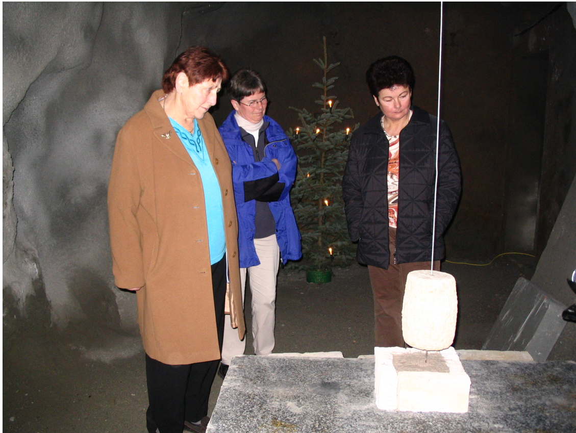
Figure 5.23: Reconstruction of the Bina vertical pendulum seismoscope.
