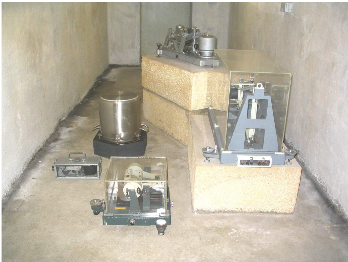
Figure 5.24: Historical instruments including Kirnos and SSJ-1,2 seismometers.
