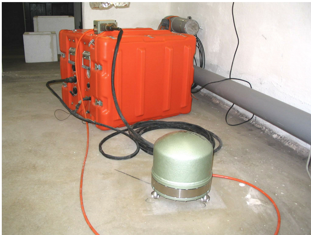
Figure 5.18: STS-2 seismometer and Quantera data logger.
