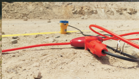
DoReMi - digital telemetry exploration seismograph
