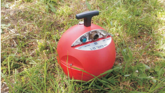
Weak motion sensor and microtremor (HVSR) Nodal systems - Terrabot
