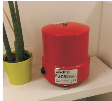
SS08 - 120"-100Hz broad band seismometer
