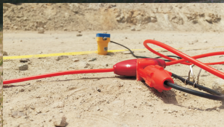
DoReMi - digital telemetry exploration seismograph
