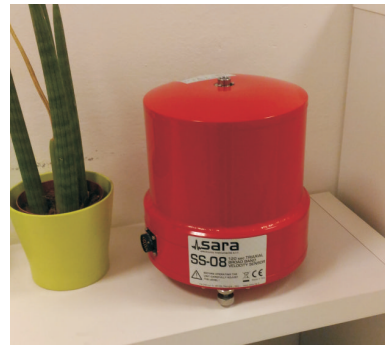
SS08 - 120"-100Hz broad band seismometer
