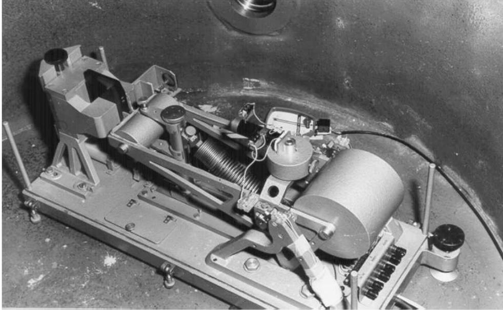
**Figure 5.7:** *Kirnos Seismometer with Plešinger's feedback loop (Photo: Plešinger)*
