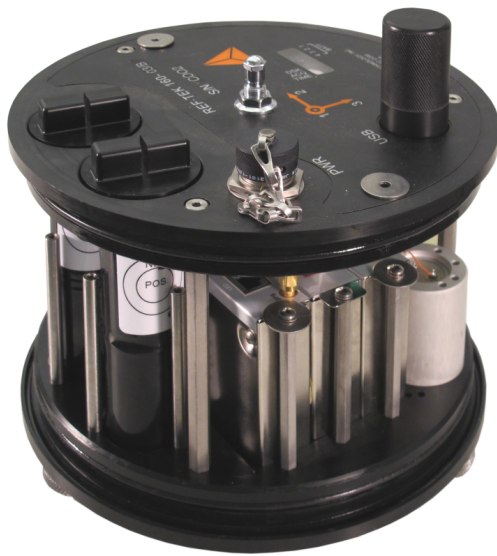
Figure 2: Inside the case of the REF TEK 160-03 High Resolution Aftershock System
